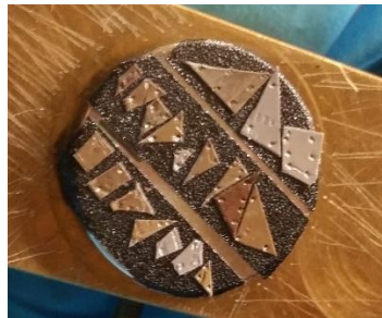
Figure 15. Membrane parts with a coat of a mixture of 40:60 of gold (Au) and Paladium (Pd)
