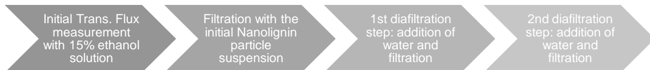
Figure 10. Diagram of the membrane filtration process for the cross-flow system.
